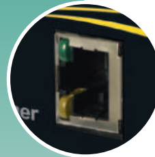
IEC 61850 server Ethernet port
